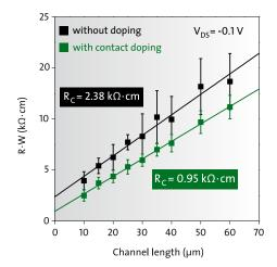
Width-normalized resistance as a function of the channel length for pentacene OTFTs with and without area-selective NDP-9 contact doping. By linear extrapolation the contact resistance (at L=0  $\mu$ m) is extracted. Transistors without doping exhibit a contact resistance of 2.38 kOhm-cm, whereas NDP-9 contact doping reduces this value to 0.95 kOhm-cm.
