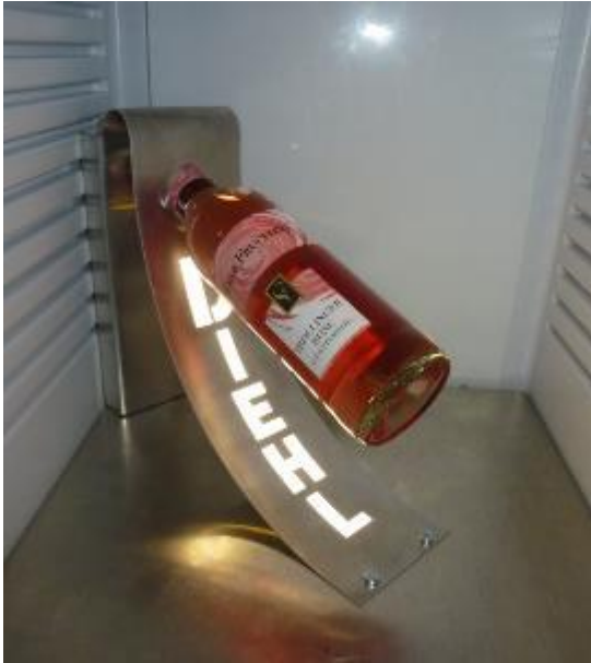
“Coolfood” OLED demonstrator from DIEHL using an OLED module fabricated by Fraunhofer FEP on flexible ultra-thin glass.
