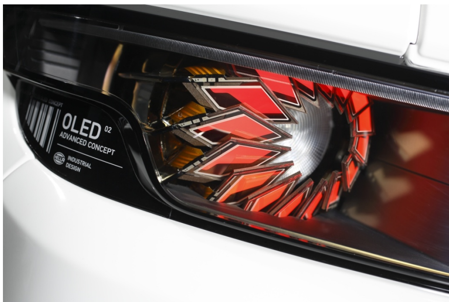
Picture 1: HELLA car rear-light based on 16 red OLEDs.
